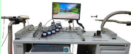
Gas Flow Meter Calibration Bench
